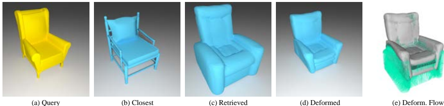
Fig. 1. Example of deformation-aware 3D model retrieval. Given a query (a), the closest 3D model in terms of Chamfer distance has distinct geometric and semantic differences. The model retrieved with our framework (c) better fits the query after deformation (d). The deformation flow is visualized in (e).
